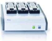
Figure 1. xCELLigence RTCA DP instrument and work station. Note that the instrument has three separate cradles, each of which holds a 16-well plate.
