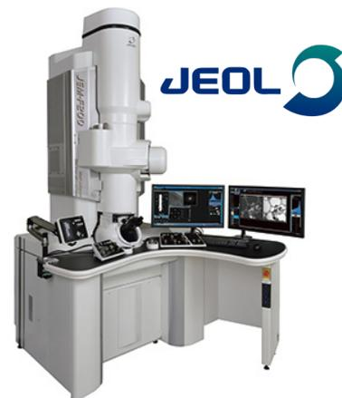
JEM-F200 field emission transmission electron microscope
