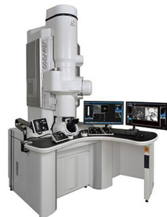
JEM-F200 field emission transmission electron microscope
